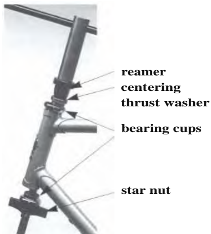
Figure 6. Head cup press assembly
