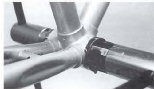
Figure 14. Reaming bottom bracket shell to remove stripped threads
