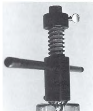
Figure 9. Fork crown race cutting
