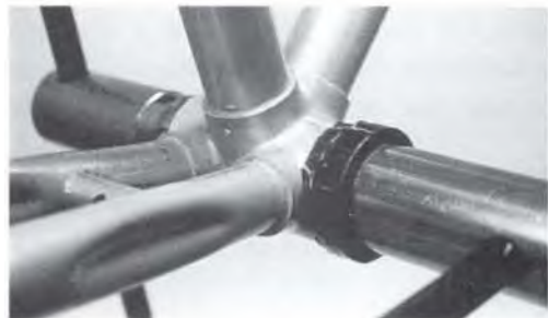
Figure 13. Milling bottom bracket face
