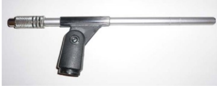
Figure 2.2.2: Measurement Microphone with DIY microphone holder
