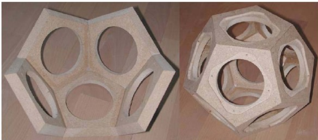
Here are two more images from the construction phase; 5/12tel dodecahedron left, to the right of final Carcass:
