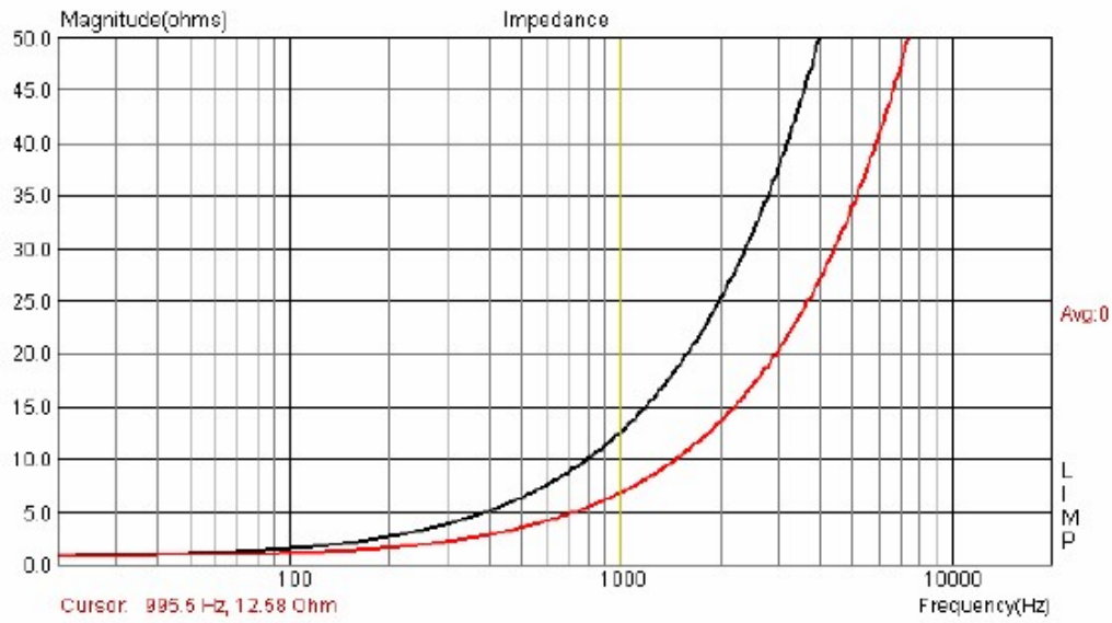
Image 5.3.2: Maximum variation range of the coil (red = no core, black core with =)
