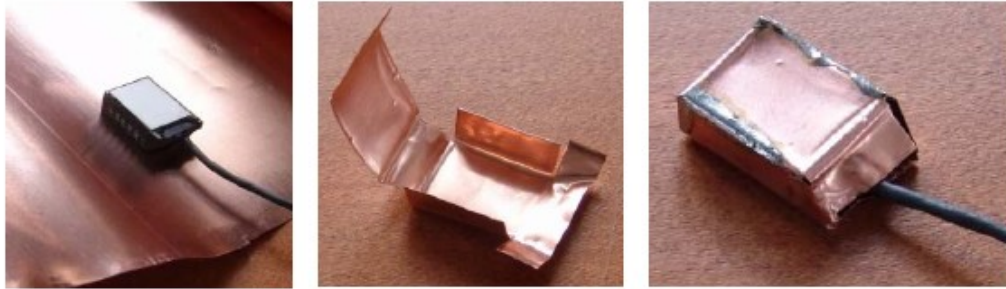
Image 2.4.3: Screening of ACH01 with copper foil
