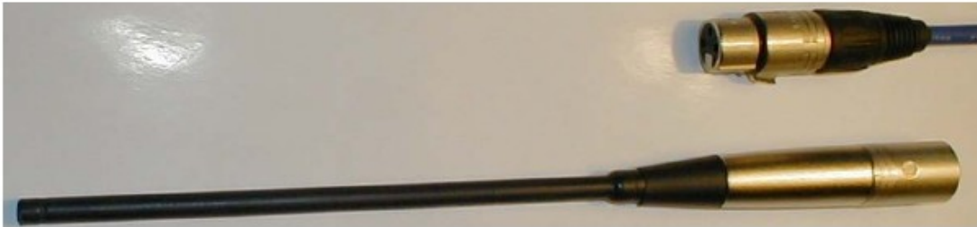
Figure 2.3.1: Finished measurement microphone (version Goran Repanić, Split)
