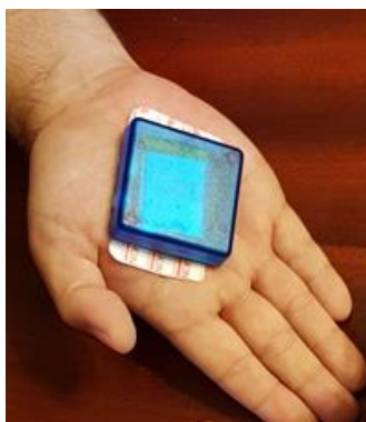
Picture 2. Open-source Bio-Monitor (OBIMON) for electrodermal measurement (K. Kasos et al., 2019) used in Study 3.
