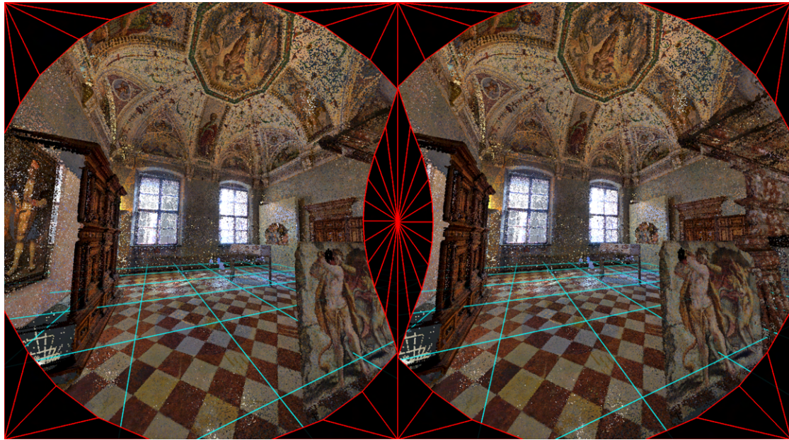
Figure 4.4: A separately rendered mesh serves as a mask to discard fragments beyond the visible area of an VR device's screens early on.
