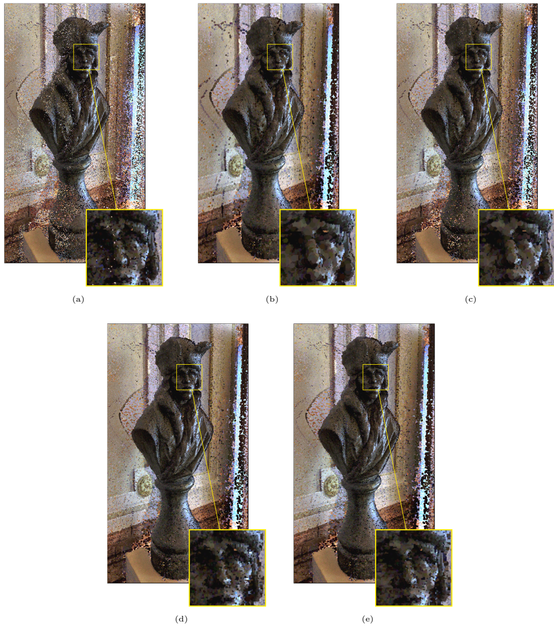
Figure 4.5: Incorrectly sized points may lead to a holey appearance (a — point size of 1px) or visual clutter (b — point size of 5px). An adaptive point size strikes a balance between both artifact types, but does not eliminate them completely (c). This can be minimized by applying paraboloid rendering (d — diameter of 5px) or filling (e — 5x5 filter kernel and point size of 1px).
