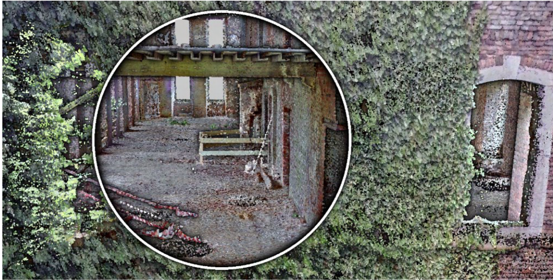
Figure 3.2: Example of a point cloud consisting of indoor and outdoor scans. It is explored with a see-through lens to inspect the occluded interior of the building in the context of the overall scan.
