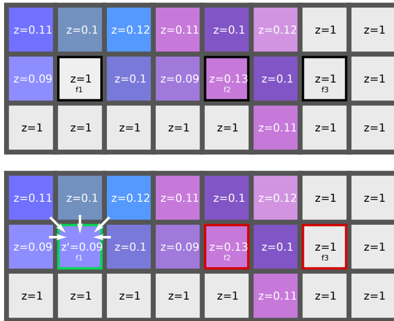
Figure 4.7: Fragment f_1 is detected as a hole based on depth differences to its neighbors and gets assigned the minimum depth value within its neighborhood; f_2 and f_3 remain unchanged as they fail the distance threshold and the minimum number of neighbors, respectively.
