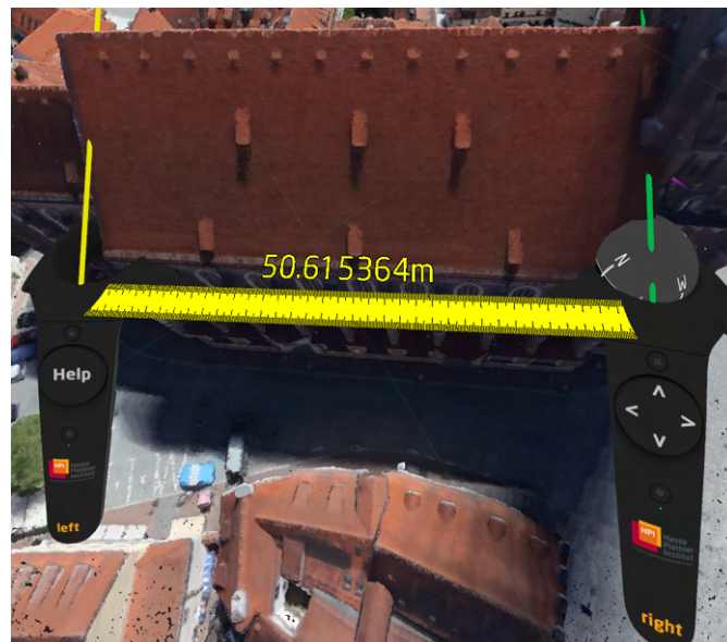
Figure 4.8: The virtual tape measure enables the user to take quick measurements in object space.
