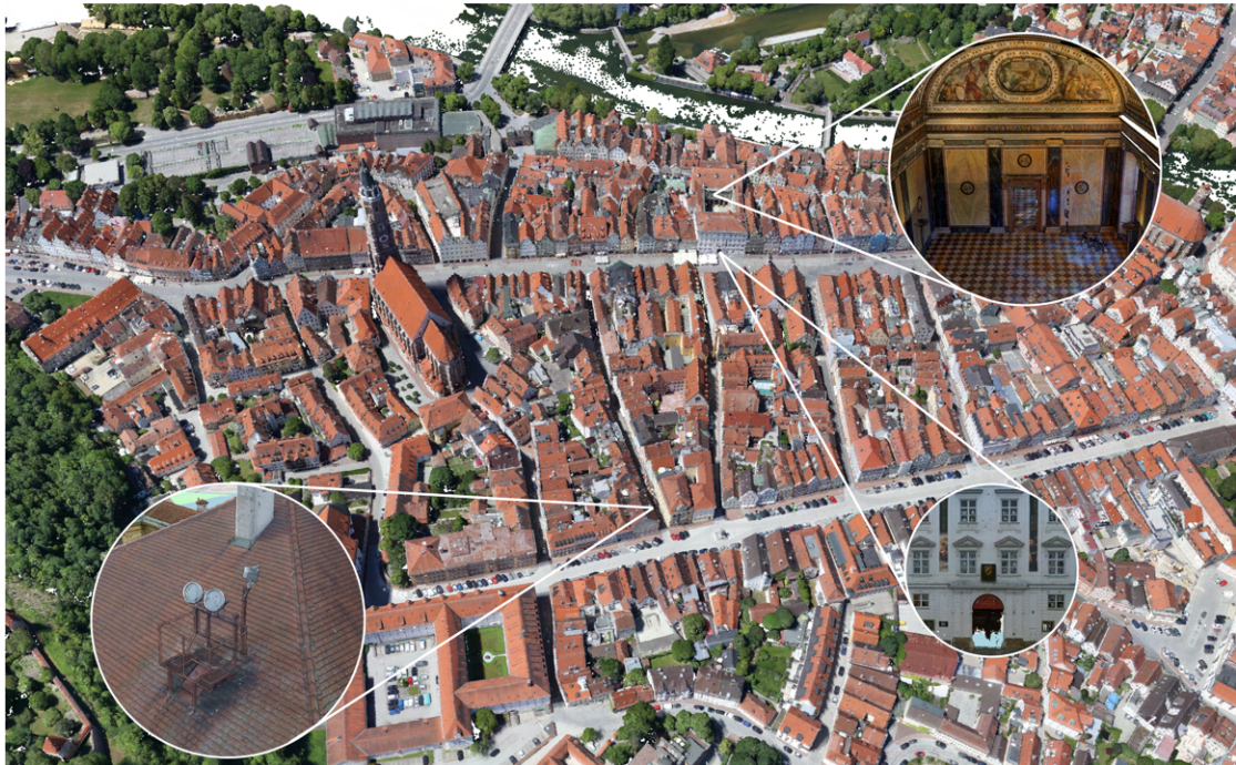
Figure 2.2: Fusion of several point clouds representing different sites and objects within the inner city of Landshut, Germany, at varying scales. Data was captured and provided by Elektra Solar and Illustrated Architecture.
