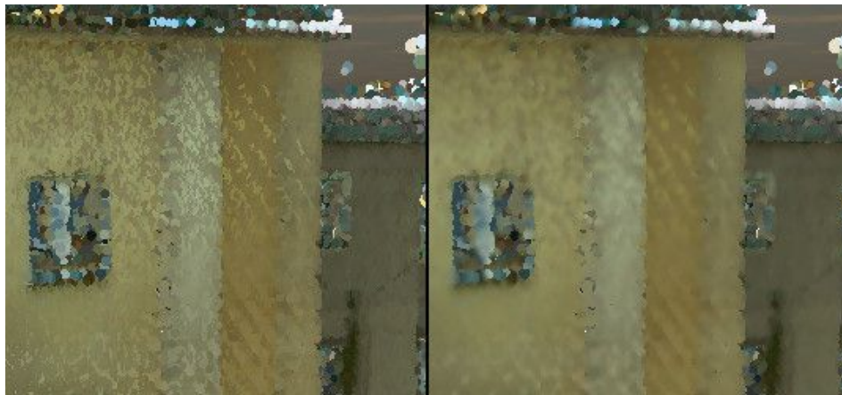
Figure 4.6: Contrasting color values can be harmonized using blurring to smooth aliasing and z-fighting.
