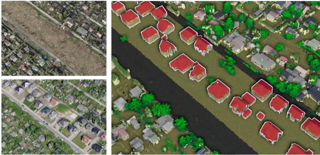
Figure 3.3: 4D point cloud enriched with surface category information: Points representing buildings that are not present in the earlier scan (upper left) but captured in the new scan (lower right) are highlighted with a red color scheme and by tracing their boundaries.
