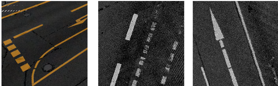
(a) Point cloud with detected road markings represented as orange shapes rendered on top of the point cloud.
