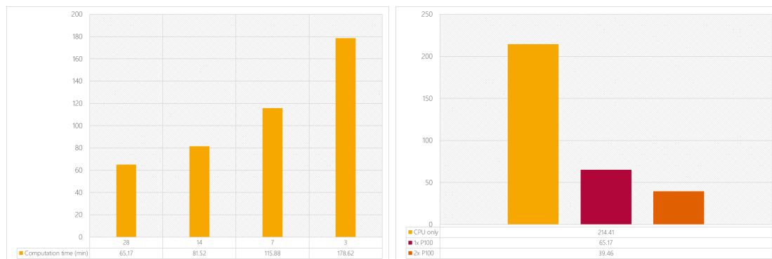
(a) Computation time in minutes of the change detection for different numbers of CPU cores used (for one GPU).
