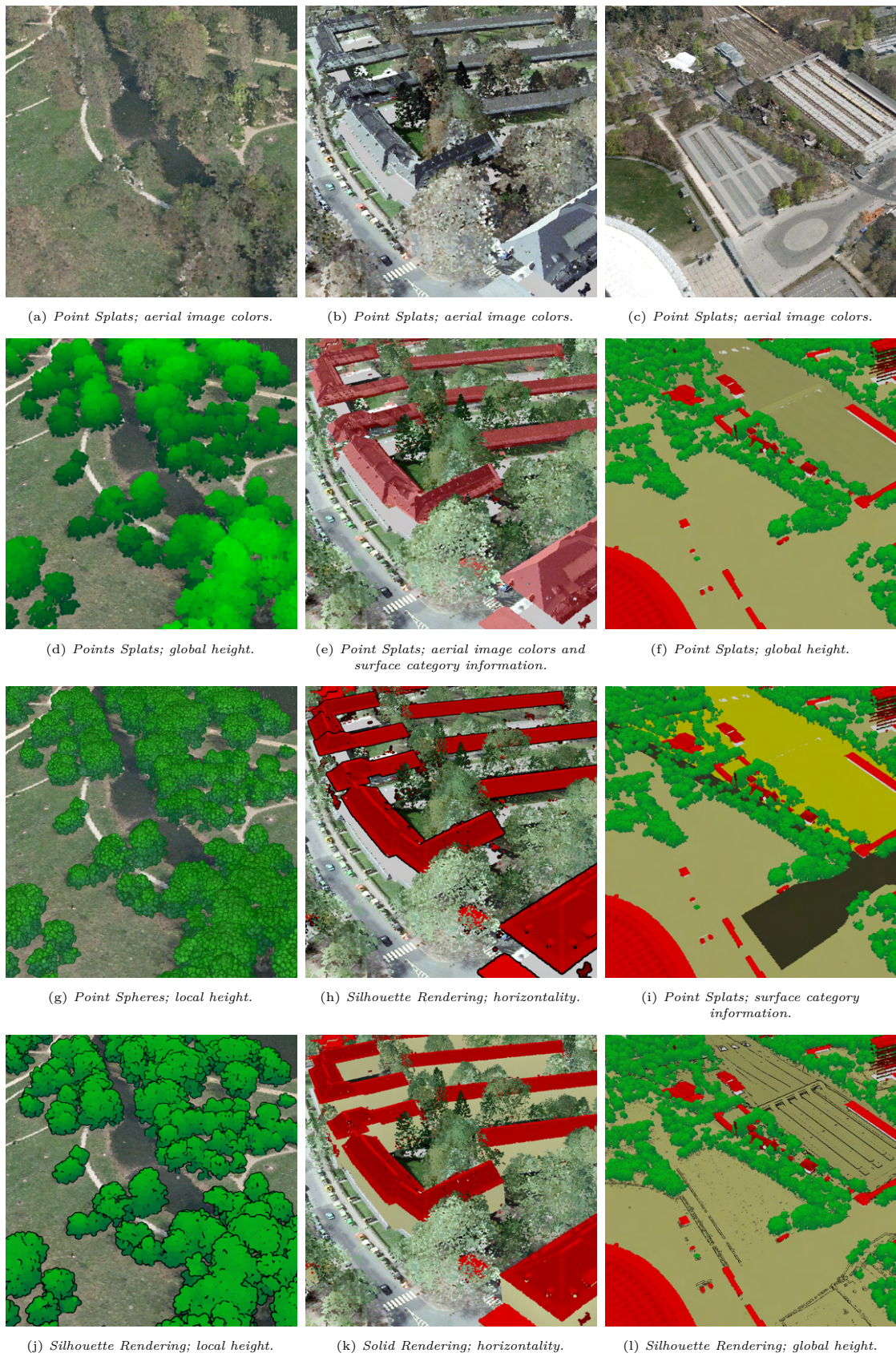
Figure 3.5: Examples of enriched point clouds rendered with different rendering setups for different surface categories: Vegetation (left), buildings (middle), and terrain (right).
