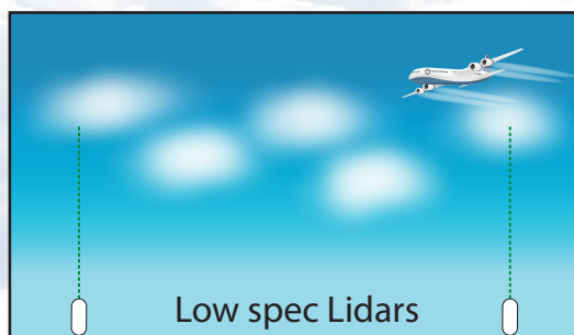
Cloud base only measured vertically by ceilometers
