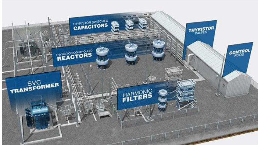
FIGURE 1.9: Typical SVC (source: GE grid solutions)
