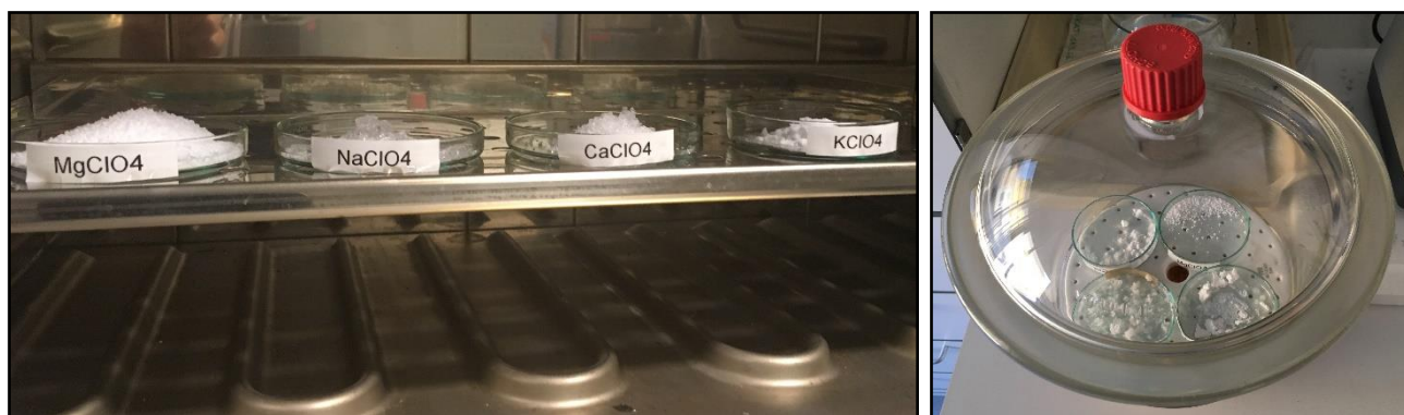
Figure 19: The perchlorate salts in glass petri dishes being placed in the incubator (Left) and desiccator (Right).
