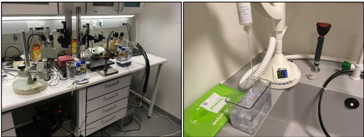
Figure 95: Both set-ups with water baths, thermometers, calibration liquids, aquariums, chambers, cold-fingers, rubber tubes, platforms, clamps, sensors, lamps, horizontal microscopes, amperemeters, A/D-converters, motor-controllers, computers and the cooling system below the table (Left). One of the water baths being filled with Ultrapure MiliQ water (Right).
