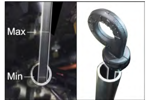
Figure: Oil level measurement on a petrol/gas engine (KM 105/... und KM 125/...)
