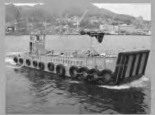
1944 56 Foot Work Boat — C51828 Hull: Steel Twin Detroit Diesel Inboard Engines
