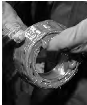
Fig. 23. Grease can easily be packed by hand.
