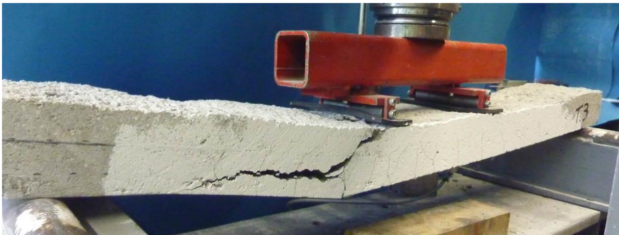
Figure 24: 3-D reinforced specimen after bending test
