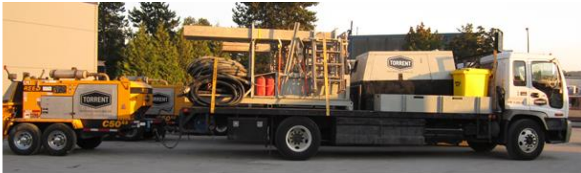
Figure 34: Typical Wet-mix shotcrete equipment set up
