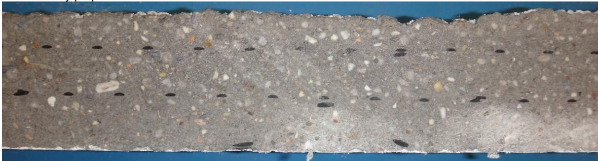
Figure 22: Cross section of system with 3-D mat
