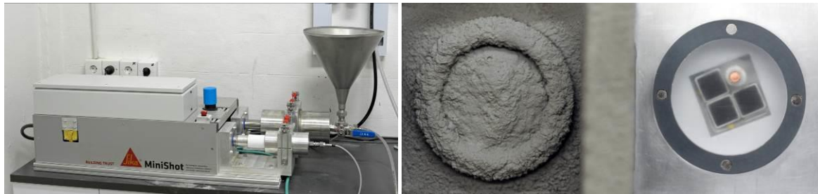
Figure 39: MiniShot-Laboratory System . Left: MiniShot spray applicator , centre: test specimen ; right: detector of ultrasound spectrometer .
