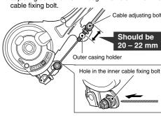
6. Check that both ends of the outer casing are securely inserted into the cable adjusting bolts of both the brake lever and brake arm.
