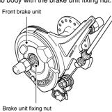
Tightening torque: 15 - 20 Nm {130 - 174 in. lbs.}
