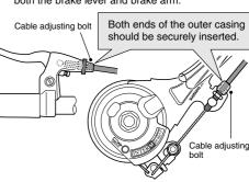
7. Push the link back until it stops. Then, while pulling the inner cable to apply the full amount of tension to the cable, tighten the inner cable fixing nut.
