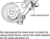
Adjusting the brake cable
