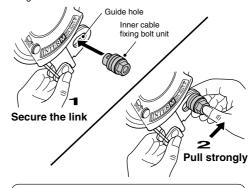
While looking from the rear of the link, check that the inner cable fixing bolt unit is firmly seated in the position shown in the above illustration.
