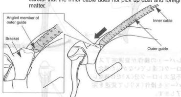
4. Set the outer casing on the inner cable, and in the bracket along the outer guide.
