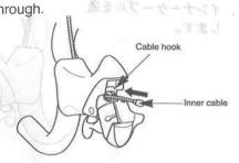
3. Fix the outer guide to the inner cable, and set the angled member in the bracket.
