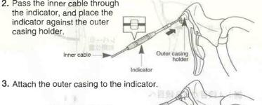
Attach the outer casing to the indicator.
