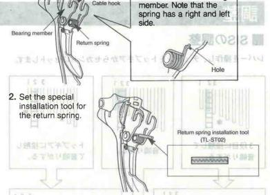
3. Assemble the bracket and lever. Be careful that the end of the return spring does not protrude from the hole in the bearing
