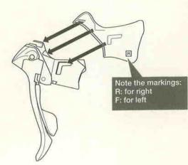
Wipe a little rubbing alcohol inside the bracket cover to make installation easier.
