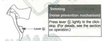
3. After trimming, adjust the gap between the chain and chain guide to the minimum setting (0~0.5 mm) using the cable stopper outer adjustment bolt.
