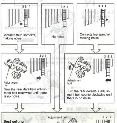
Turn the crank forward while turning the rear derailleur adjustment bolt slowly counterclockwise. Stop just before noise is produced (the chain contacts the third sprocket)
