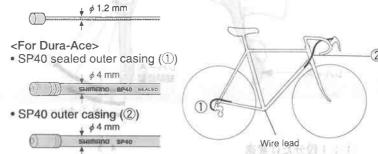
Inserting the inner cable
