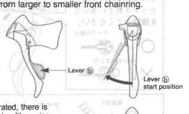
When lever (b) is operated, there is one click where trimming (the noise prevention mechanism) engages, and a second stronger click when the gear shift stroke is completed. After trimming, the next push will complete the gear shift stroke to the smaller front chainring.
