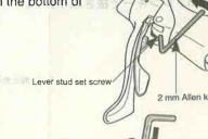
2. Insert a 25 mm Allen key or similar tool into the lever stud hole, and tap it gently with a plastic mallet to push out the lever stud. When the lever stud comes out, the bracket body and lever body can be disassembled.
