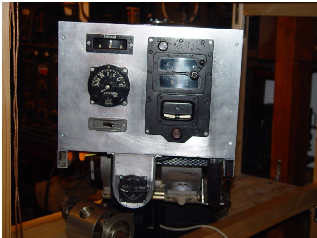
Figure 32: Instrument panel of the LZ12 autopilot model
