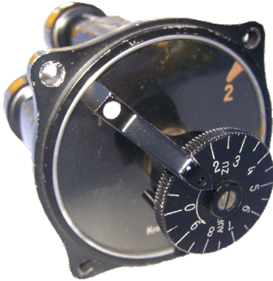
Figure 25: Lv 194 "Umschalhahn" pneumatic controller
