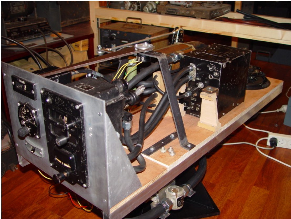
Figure 31: The complete system mounted on the turn table. The “rudder” on top is coupled to the drive system of the the turn table so that the LZ12 controls the movement of the turn table.
