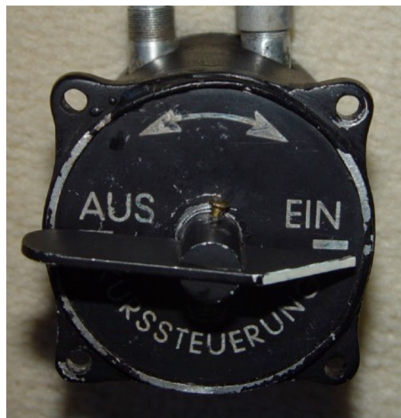
Figure 26: Lzr 4r "Hauptschalter" main operating switch
