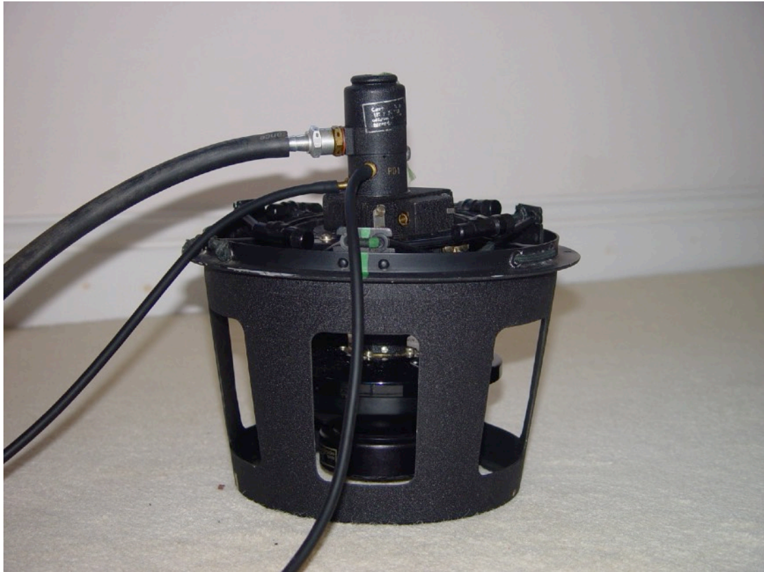
Figure 6: Complete Lfk 9 Master compass fitted with protective housing and compensation ring
