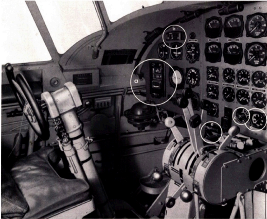
Figure 27: Cockpit overview with controls for the Lz 12 autopilot
