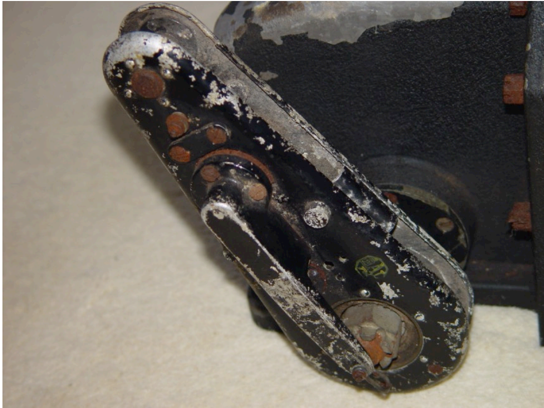
Figure 22: Close up of the output lever with the emergency release lever
