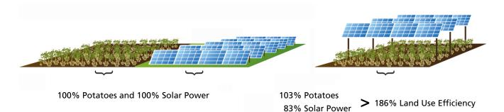
Figure 13: Through the combined use of land, the land use efficiency with agrivoltaics on the test site in Heggelbach is up to 186 percent. (Illustration of potatoes © HappyPictures/shutterstock.com)
