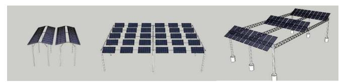
Figure 43: Illustration of different types of agrivoltaic systems with east-west, south- and south-east orientation. © Fraunhofer ISE
