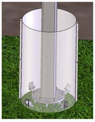
Figure 20: Fenders on the supports of the system in Heggelbach protect against damage from farm machinery. © Hilber Solar
