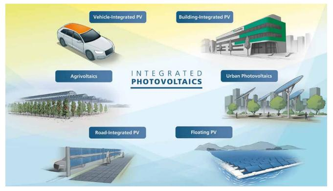
Figure 6: Applications for the integration of photovoltaics. © Fraunhofer ISE
