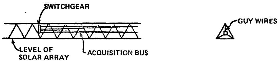
Figure 1.1.4-9 Acquisition Bus and Switchgear Support
