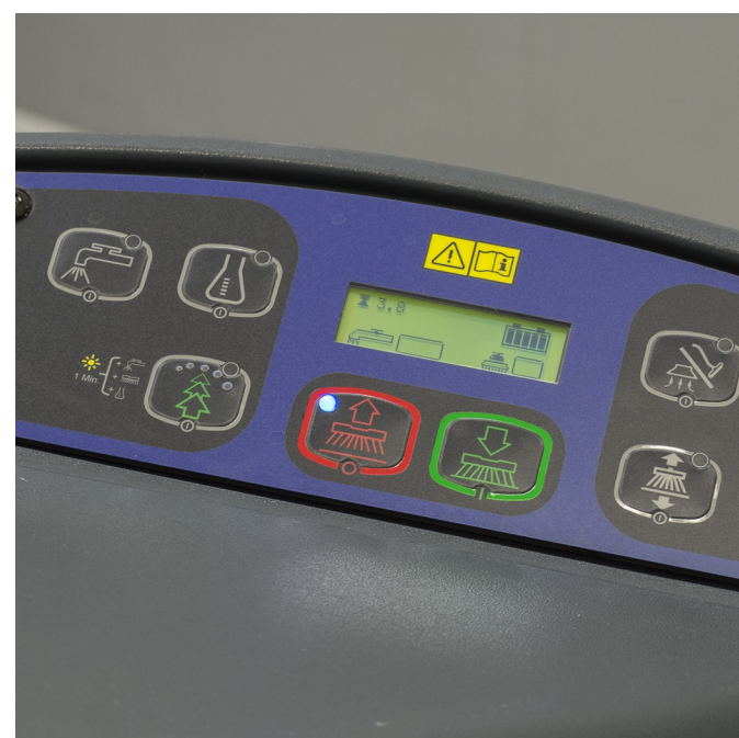
2 Check if there isn't any brush motor overload i.e. 3 battery Ledflash simultaneously.
