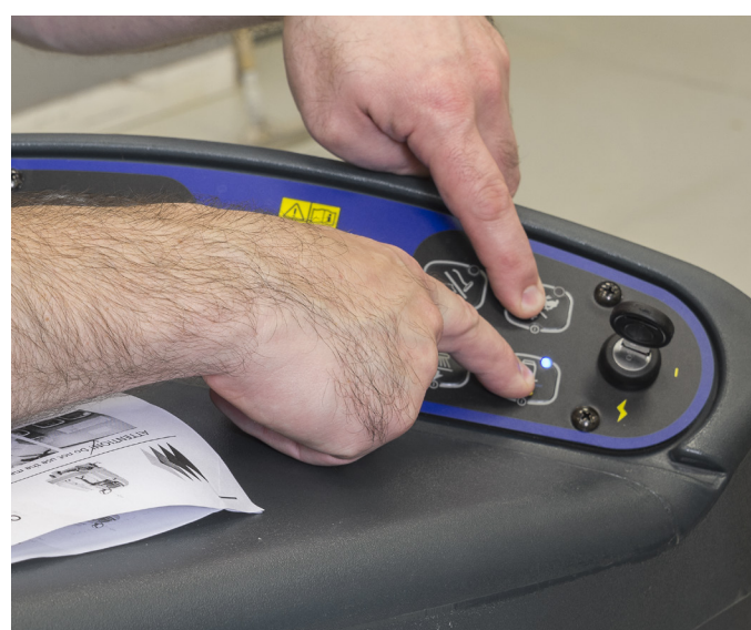
16. In case something does not work enter the Service test mode by pressing the Speed switch and the traction control switch, then on the key. Go through the menu.
