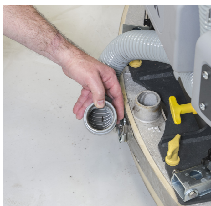
1 Check if the suction hose is correctly installed and cleaned.
