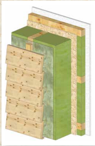
Example: External wall 1 (vapour-permeable structure)
