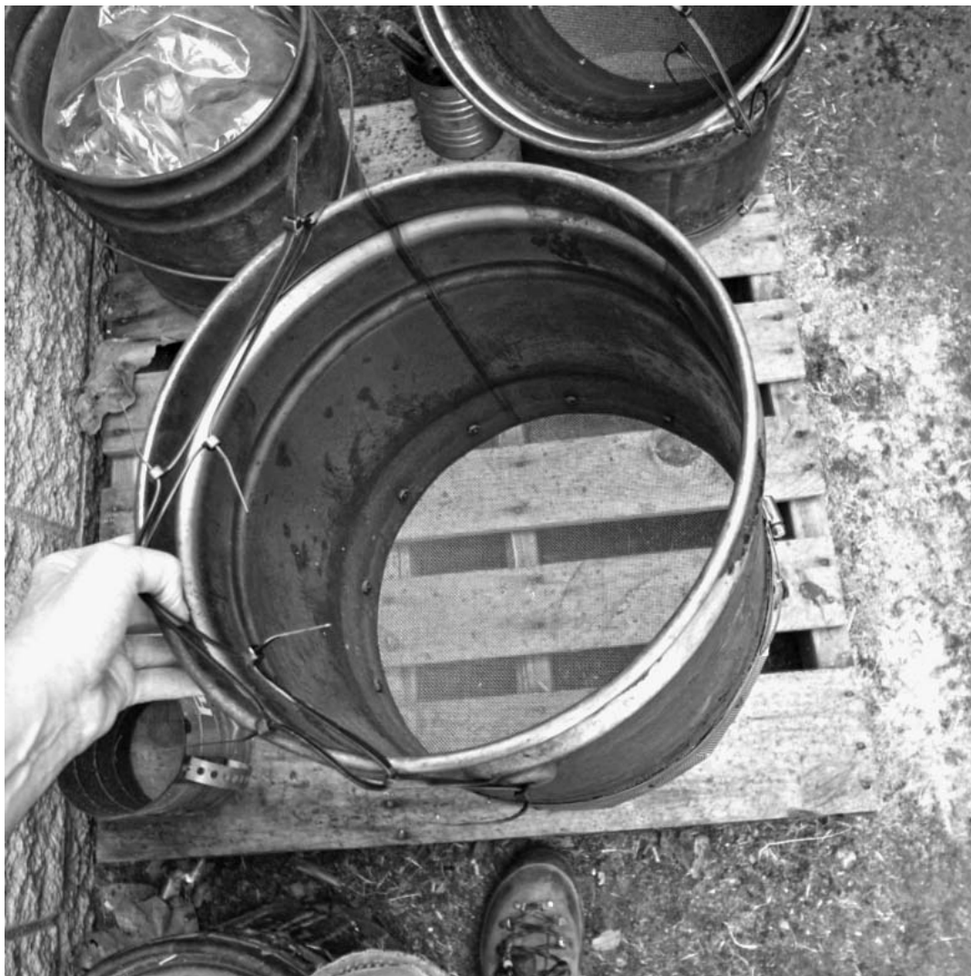
Figure 2 Five-gallon metal-screened bucket is constructed by removing the bottom of the bucket and attaching stainless steel 20-mesh screen with machine screws and a large-diameter hose clamp.
