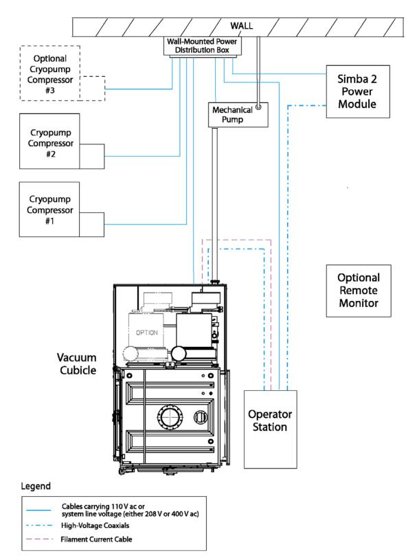
Figure 3-8 Routing of Electrical Power Cables on Simba 2-Powered Systems
