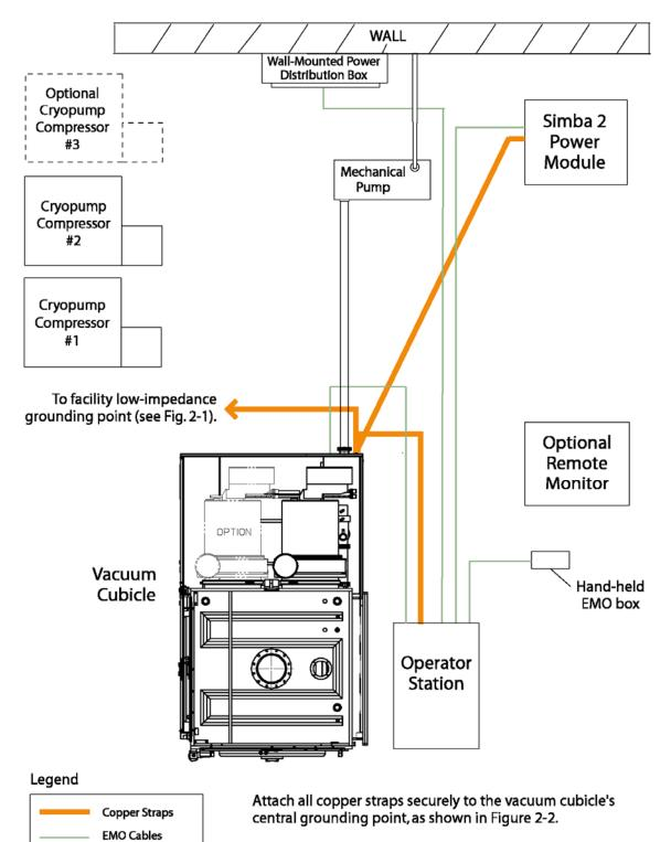
Figure 3-9 Routing of EMO Cables and Copper Straps on Systems with the Simba 2 Power Supply
