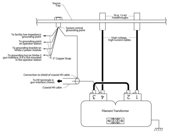
Figure 2-2 Vacuum Cubicle Grounding for Simba 2 Power Supply
