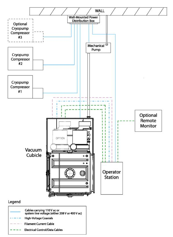
Figure 3-10 Routing of Power and Control/Data Cables on Systems With Either the CV-6SLX or the CV-12SLX Power Supply
