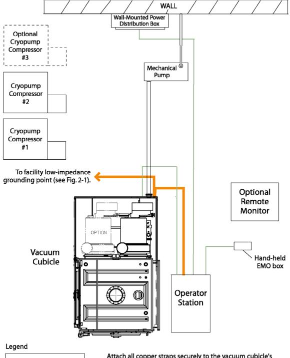
Figure 3-11 Routing of EMO Cables and Copper Grounding Straps on Systems With Either the CV-6SLX or the CV-12SLX Power Supply
