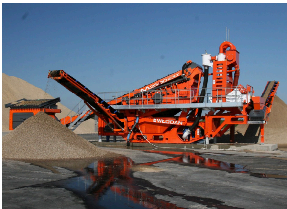
Figure 4: Mobile washing plant for treating contaminated soils and sediments. Source: https://www.flickr.com/photos/marine_corps/8413440131/
