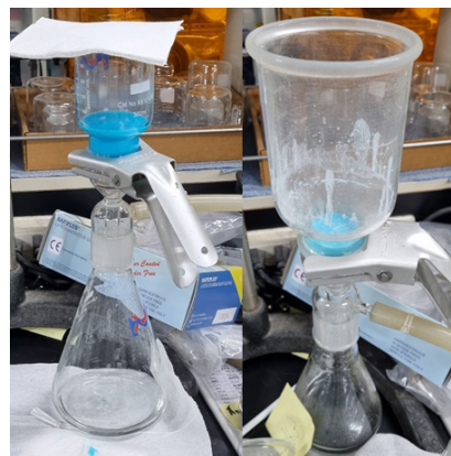
Figure 2: Experimental setup of the vacuum filtering procedure after HKUST-1 synthesis.
