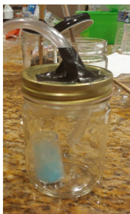
Figure 3: Experimental setup of the CO 2 adsorption process.
