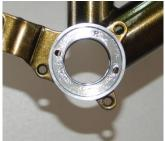
1) Screw the steel bottom bracket caps firmly into the frame by using the special EX-Tool. Make sure the tool fits firmly to the ground of the cap. Torque: 40 Nm.
