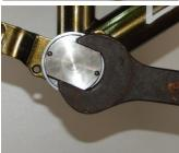
NOTE: Watch the screwing direction! Left side: right-hand-thread ("R"); Right side: Left-hand thread ("L")
