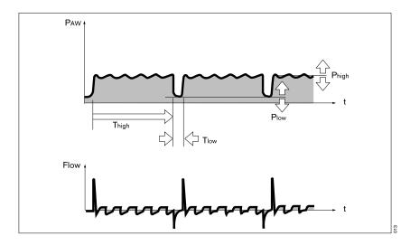
Set the pattern of ventilation for APRV with the ventilation parameters:
