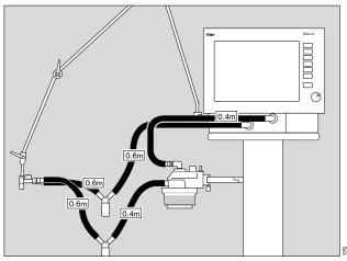
Always hold the hoses by the connection sleeve and not by the spiral ribbing when removing and connecting the ventilation hoses,
