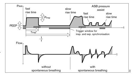
Set the pattern of ventilation for BIPAP and BIPAP/ASB with the ventilation parameters:
