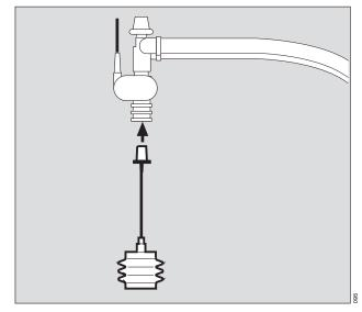
Switch on unit = pivot flap\* upwards and press power switch until it clicks into position. The flap falls over the button to protect against inadvertent switching off.
