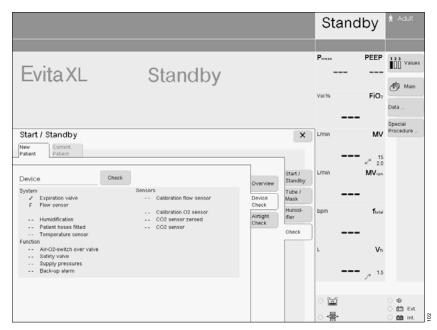
A device check cannot be performed during automatic calibration of the flow sensor or O2 sensor:
