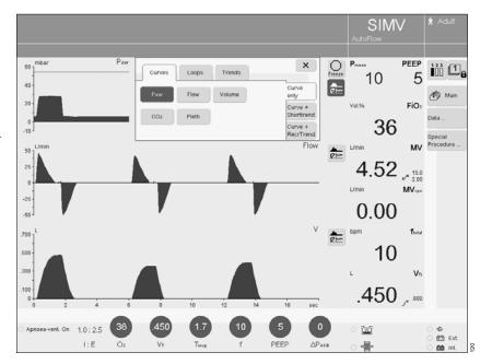
EvitaXL displays the short trend of the associated parameter over the last 20 minutes on the left, beside the real-time curve.
