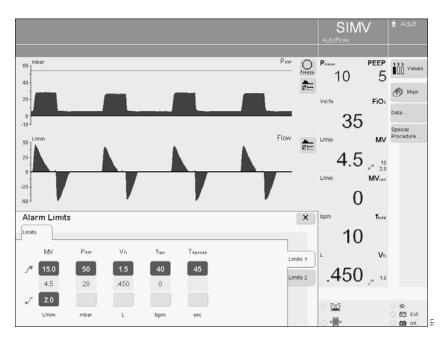
The alarm limits for the optional measured value etCO<sub>2</sub> can be viewed by touching "Limits 2".
