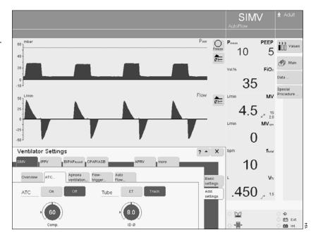
Activated tube compensation is indicated by EvitaXL by the tube symbol and tube diameter in the status line.
