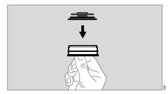
Insert stopper with diaphragm on top into the housing from below and screw in tightly.
