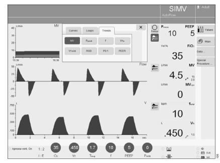
Touch the required parameter key and EvitaXL displays the trend during the last hour for the selected parameter.
