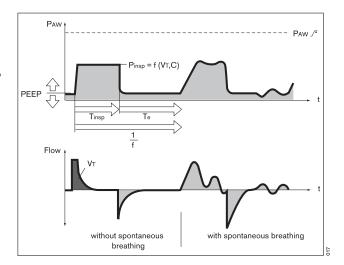
This effect can also be caused during ventilation, e.g. due to a build-up of secretion. In this situation, the pressure is limited by the alarm limit »PAW /T«. The pressure rise stops 5 mbar below the alarm limit »PAW /T«, and the alarm »Volume not constant« is only given when the set tidal volume VT is not longer applied.
