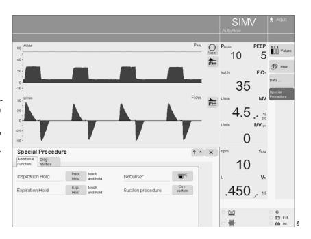
EvitaXL ventilates the patient in the set ventilation mode with increased O2 concentrations: In adult mode, the O2 concentration is 100 % by volume. In paediatric mode, the enriched concentration is 25 % higher than the set O2 concentration. If PEEP is not set to more than 4 mbar, PEEP will be applied automatically at 4 mbar. This PEEP allows EvitaXL to detect any subsequent disconnection.
