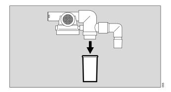
The expiration valve is only dismantled if severely soiled:
