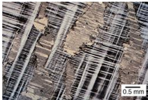
Exsolution of albite patches in microcline crystal to form perthitic texture.
