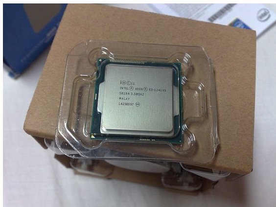
Intel Xeon E3-1241 v3 CPU, sitting atop the inside part of its retail box that contains an OEM fan-cooled heatsink
