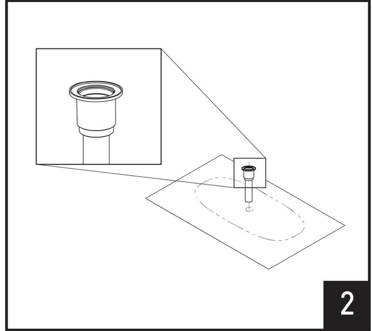
Install bathtub K36E/K40E waste drain into floor surface. Note the inset diagram for waste drain measurements.
