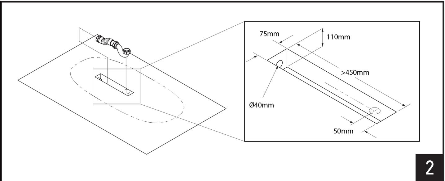
Install bathtub K12 waste drain into floor surface. Note the inset diagram for waste drain measurements.
