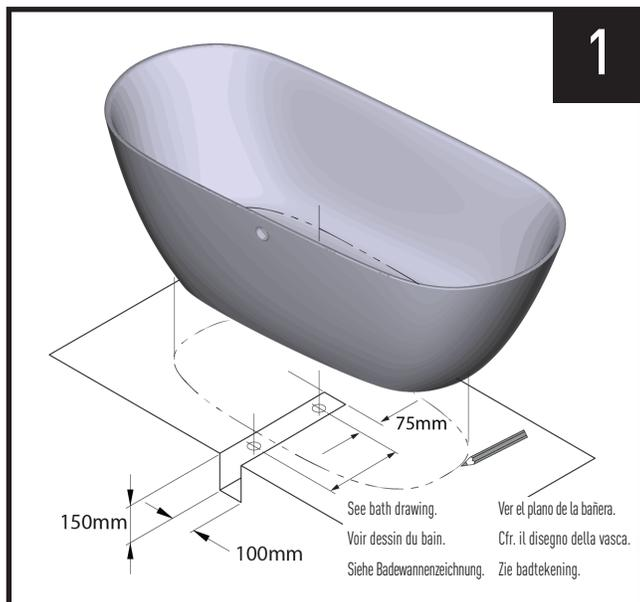
Measure bathtub diameter and mark accordingly on floor surface for appropriate waste drain installation connections.
