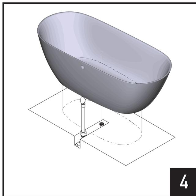
Position bathtub so the drain holes are aligned.
