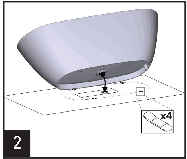
Position the bathtub spacers (x4) as shown and ensure bathtub drain hole is aligned with waste drain before positioning bathtub.
