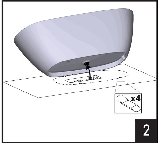
Position the bathtub spacers (x4) as shown and ensure bathtub drain hole is aligned with waste drain before positioning bathtub.
