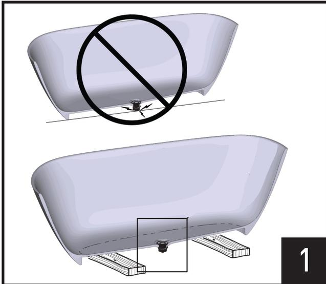
Ensure bathtub is supported by 2x4s to not damage the drain. See K36E/K40E drain instructions for installation.
