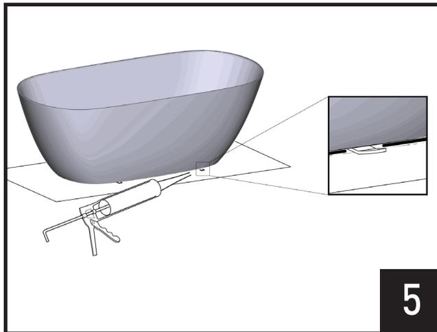
Apply silicone sealant along bathtub edge footer. Do not seal over bathtub spacers.
