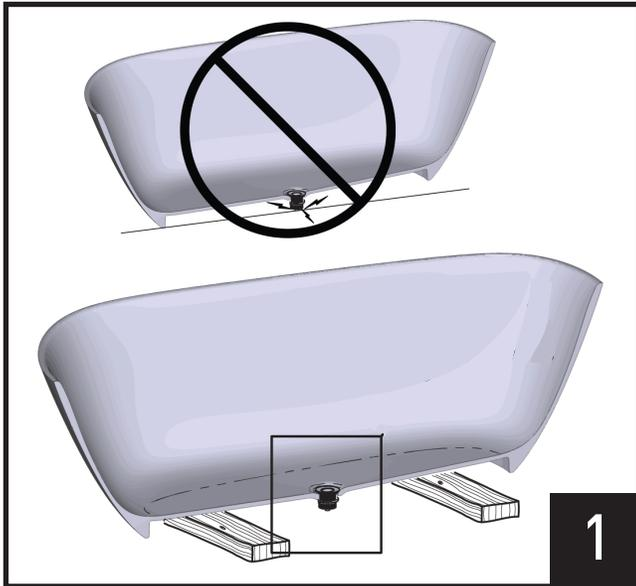
Ensure bathtub is supported by 2x4s to not damage the drain. See K36/K40 drain instructions for installation.
