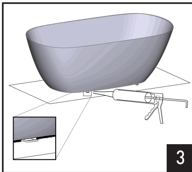
Secure top bathtub drain to bathtub. Apply silicone sealant along bathtub edge footer. Do not seal over bathtub spacers.
