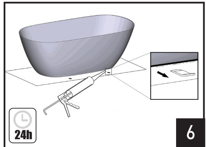
After removing bathtub spacers, apply silicone sealant (not provided) in the gap. Wait **24 hours** for fully sealed.
