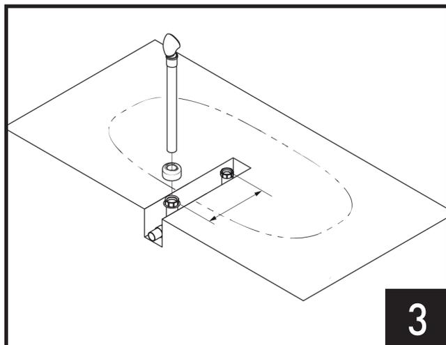
Make appropriate drain fitting connections. (See bath drawing).
