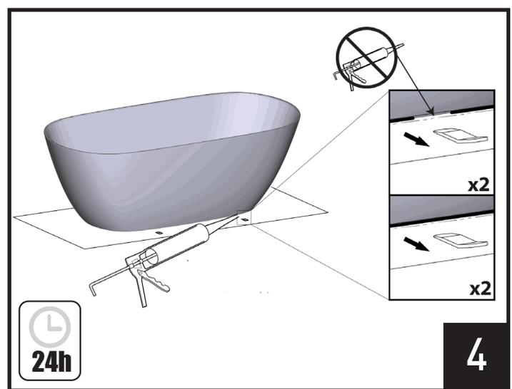
After removing bathtub spacers, apply silicone sealant (not provided) in the gap. Wait **24 hours** for fully sealed. Installation complete.
