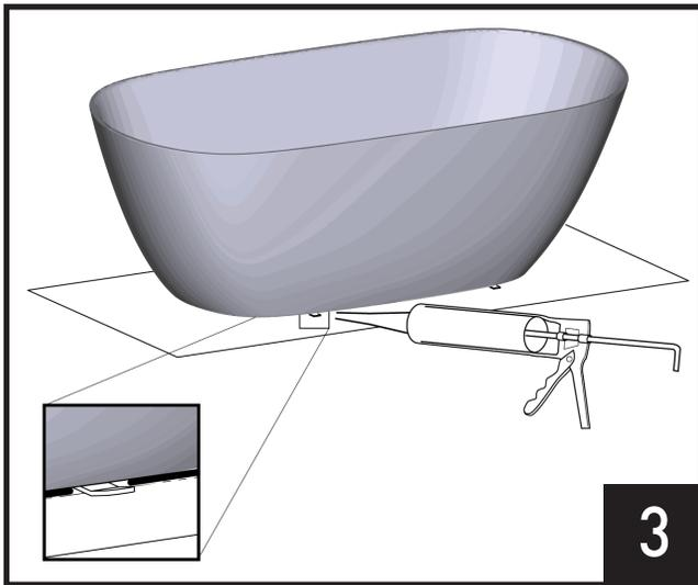
Secure top bathtub drain to bathtub. Apply silicone sealant along bathtub edge footer. Do not seal over bathtub spacers.
