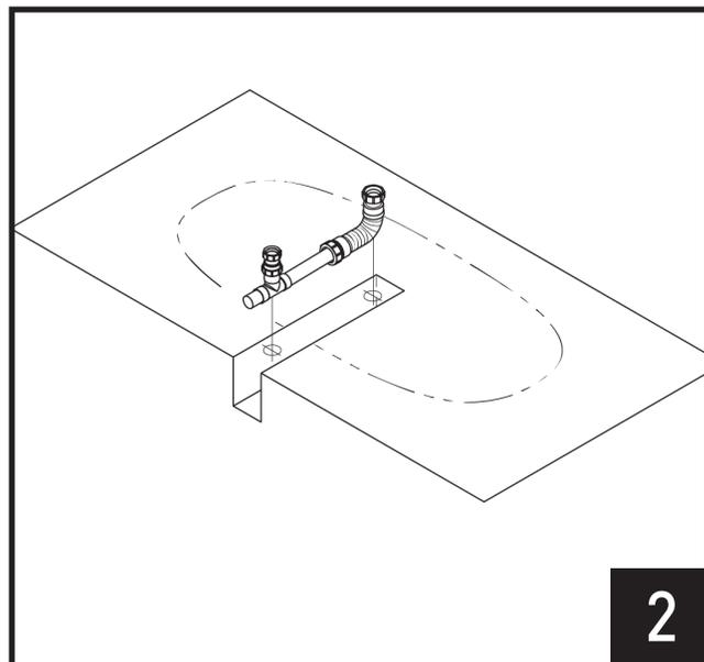
Install either K17 or K51 bathtub waste drain within floor surface.
