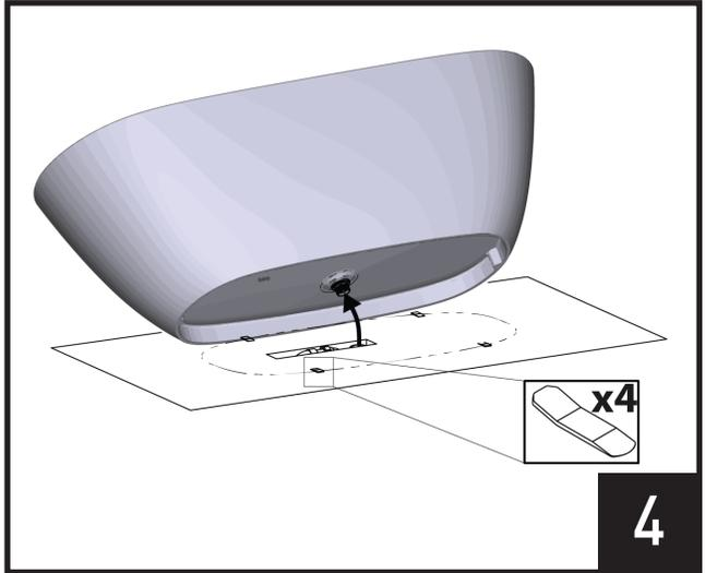
Position the bathtub spacers (x4) as shown and ensure bathtub drain hole is aligned with waste drain before positioning bathtub.
