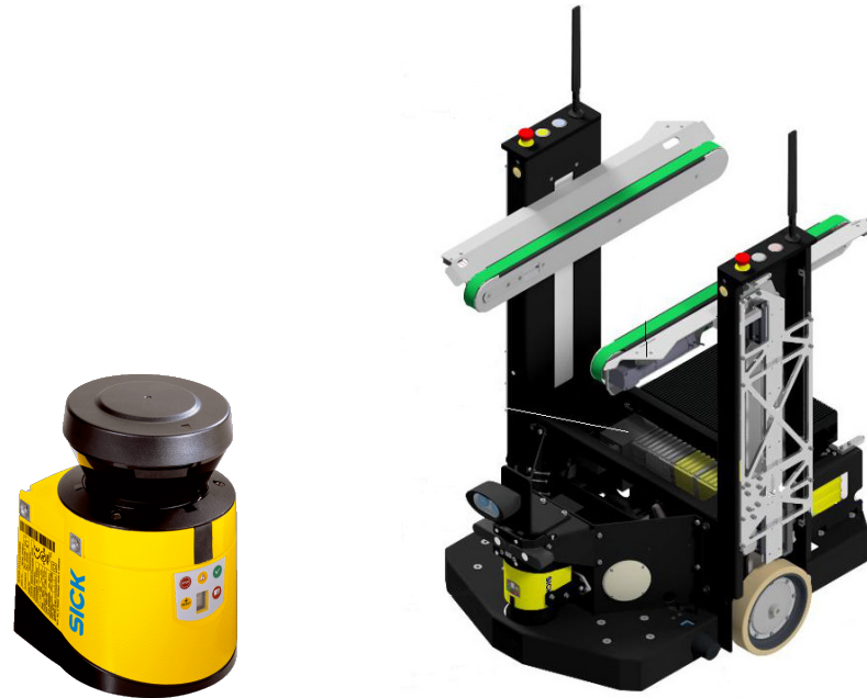
Figure 3.10: SICK 300 laser scanner (left) installed on the proANT 436
