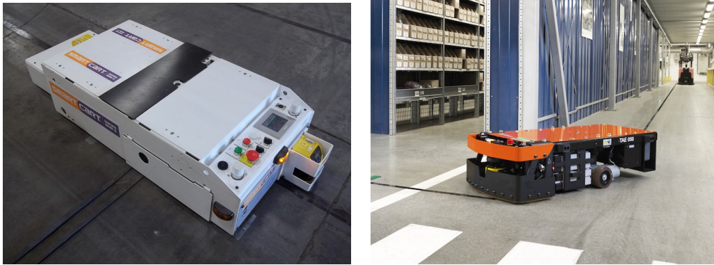
Figure 4.11: On the left a SmartCart 100 ST-R and on the right a Toyota TAE050, both magnetic guided AGVs that use a laser scanner for personal safety.
