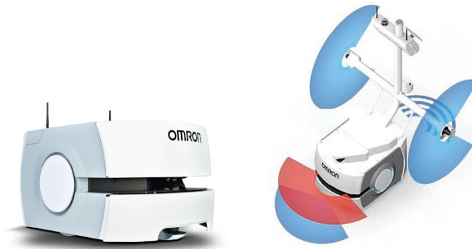
Figure 4.8: Omron LD Platform, a very flexible vehicle featuring different interesting sensor solutions.
