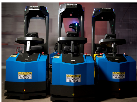
Figure 4.4: Seegrid GT10, manual and automated guided vehicle allows great flexibility in warehouse facilities.
