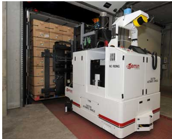
Figure 4.2: Egemin ATL, with additional scanner on top to secure the whole load/unload area.
