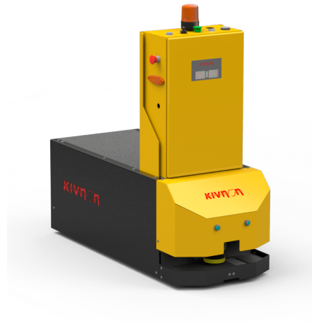
Figure 4.7: Kivnon K32 with one laser scanner in front.
