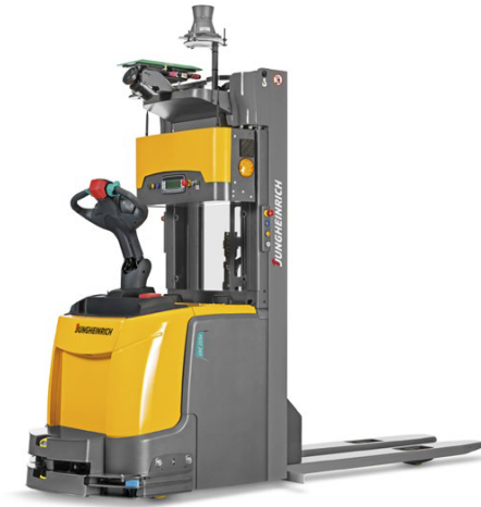
Figure 4.1: Jungheinrich ERC 215a carries a maximum payload of 1500kg and it's equipped with two Sick S3000 laser scanners, in the front and back of the vehicle.
