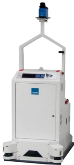
Figure 4.6: AGVE A2 with two laser scanners to secure the front and the sides of the vehicle.
