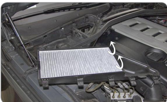
(EN) Take out the filter with its frame, remove the old filter from the frame and put in the new one. Repeat the actions for the filter on the driver's side
