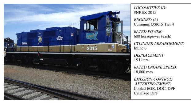
Figure 1 - Unit #2015 - NR156 2GS12B Tier 4 Locomotive
