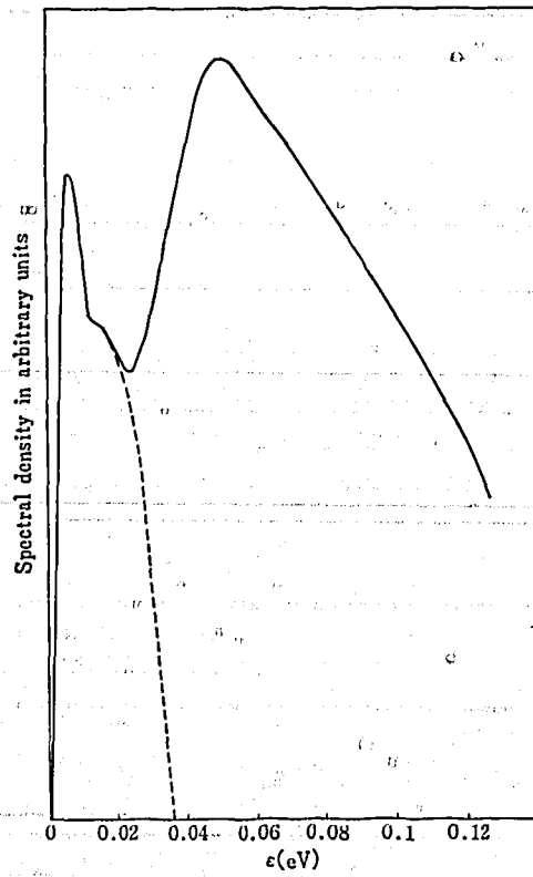
Fig. 1 Spectral density function for D_2O liquid for T=290^{\circ}K^{(1)} . (Dotted line shows the estimated \rho_{vv}^{ac}(\omega) )
