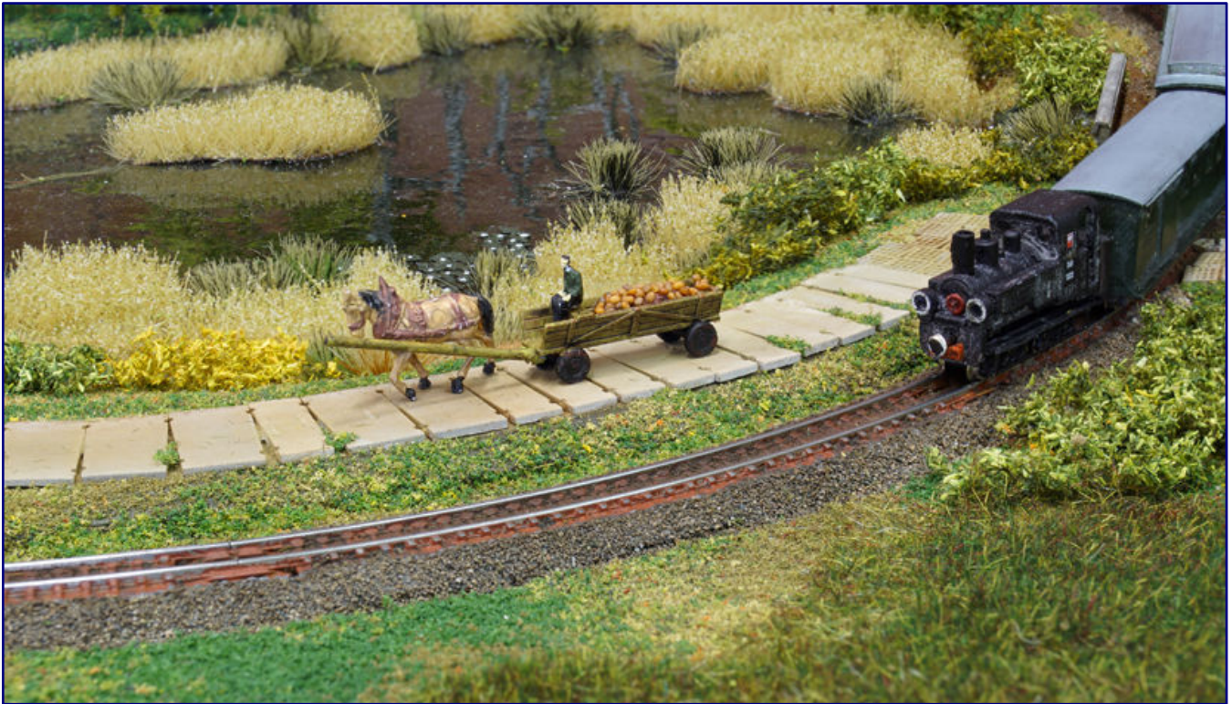
Pawel Zygarlowski's field railway runs on T-gauge tracks, but all the vehicles are self-constructed and 3D-printed. The steam locomotive with the large lanterns that were once so typical for Poland does not have its own drive. This is in the ghost car behind it in this case.
