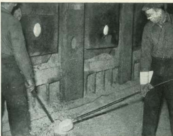
Taking a test spoonful of metal at the open hearth.
