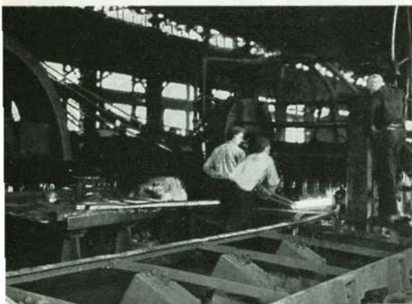
Rolling a tube after piercing. This tube is entering the final pass.
