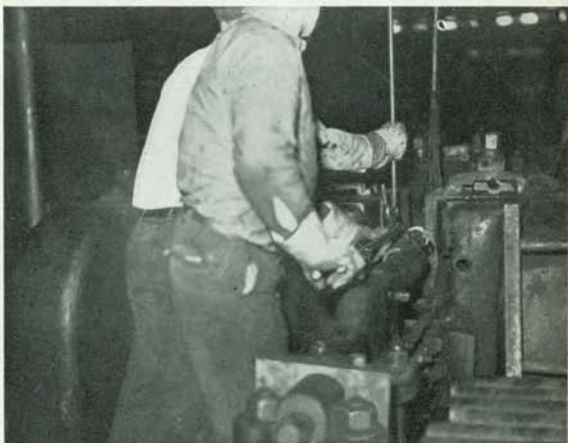
Upsetting mechanical tubing in the Specialty Department, Monessen Works.
