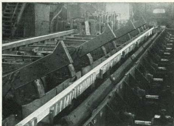
Billet mill at Monessen Works. Either round or oblong billets can be rolled here.
