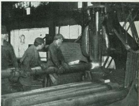
Pointing for the cold-draw dies.
