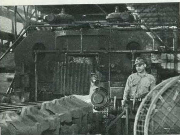
Piercing billet at the Elongator Mill. This is the outlet side of the mill.
