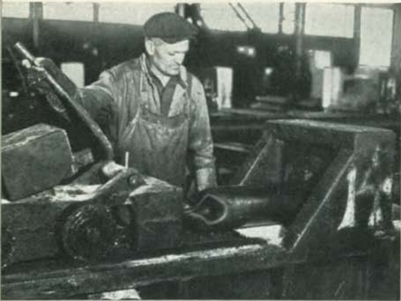
Cold drawing large-size pipe for extreme accuracy. The pipe is pulled very slowly but with great force through the die opening.
