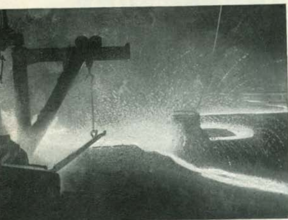
Tapping a blast furnace. The stream at the right is slag. The long white stream is iron.
