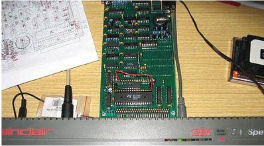
MB02+ with 512 KB single chip SRAM connected to a +2
