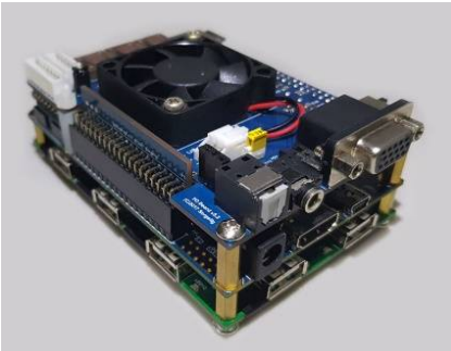
MiSTer complete configuration with daughter boards and cooling fan
