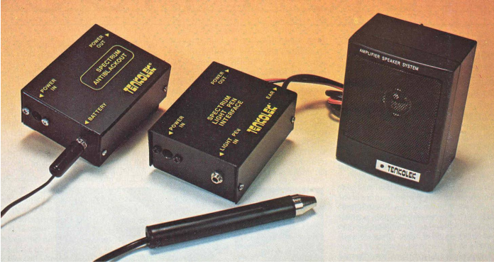
Tenkolek peripherals. Left to right: anti-blackout, light pen, sound box.
