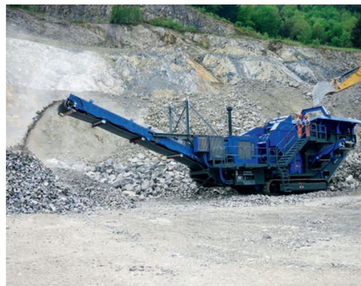
Raupenmobiler Backenbrecher Tracked jaw crusher
