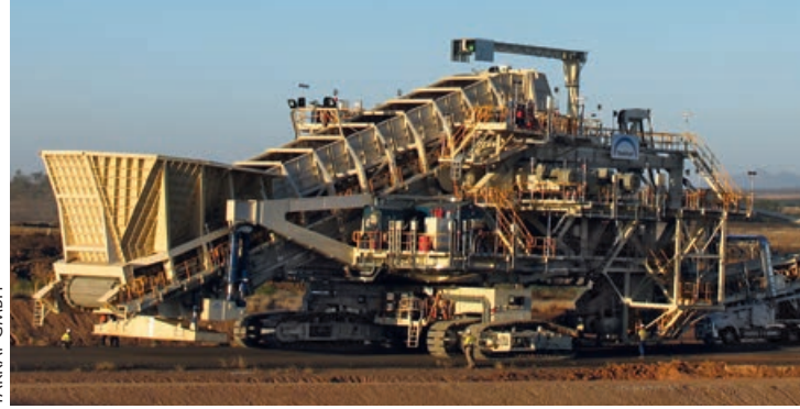
12,000 t/h mobile Brechanlage in Australien 12,000 t/h mobile crushing plant in Australia
