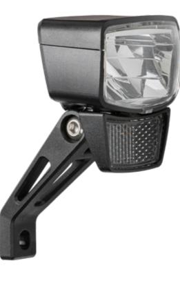
The new fork bracket is a perfect design match for the new AXA light design, making sure the light will look well integrated to the bike. The product design is also very well suitable for handlebar mounting via faceplate solutions or handlebar brackets.
