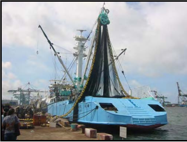
Fig. 2. Example of an advanced fishing vessel used for distant water fisheries with a 1.2 km long purse seine that can cover an area of 400 m 2 . It is equipped with a helicopter that can facilitate searching for tuna, and with a deep freezer to preserve the tuna at < -60°C.
