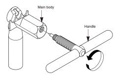
2. Remove the holder from the handle, and then take out the pin.
