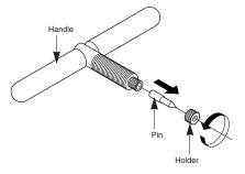
3. Remove the stopper screw from the base of the grip, and then take out a spare pin.
