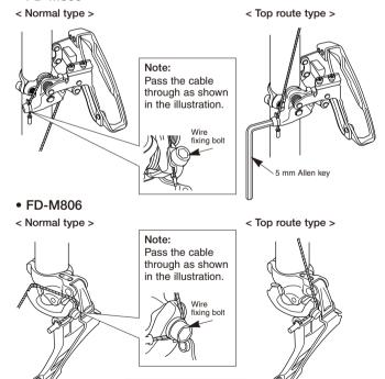
After taking up the initial slack in the cable, re-secure to the front derailleur as shown in the illustration.
