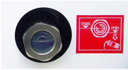
Picture 2 - Sight-glass for compressor oil
