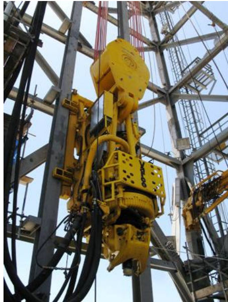
Abb. 6.24: Top-Drive-Antrieb (Thue Drilling 2007)
