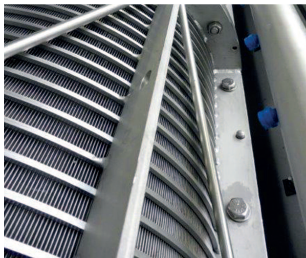
Sturdy wedge wire basket made of stainless steel
