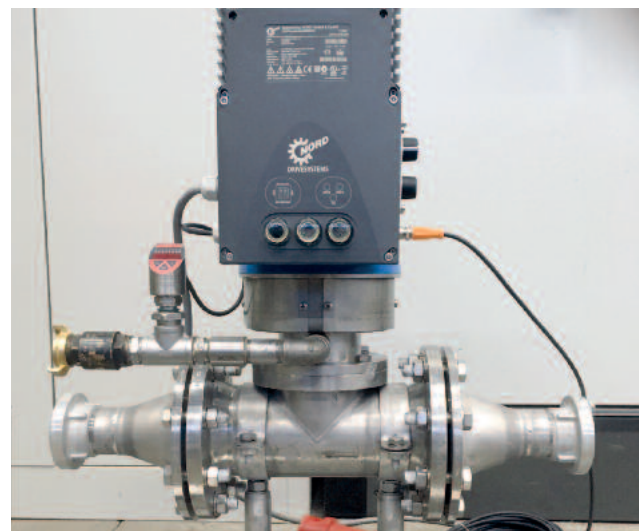
Mobile test unit of a HUBER Inline Polymer Mixer IPM
