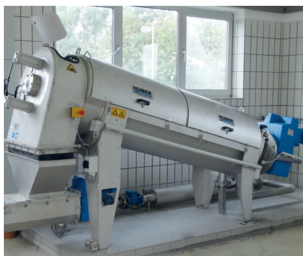
Stationary mounted screw press for 140 kgDS/h
