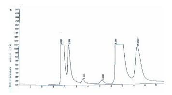
Figure 1 Ion chromatogram of toothpaste sample solution
