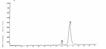
Figure 2 Ion chromatogram of strontium standard solution
