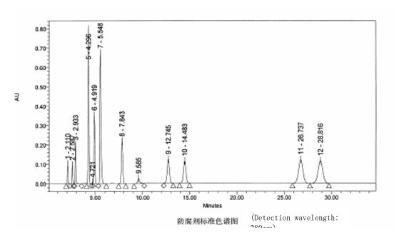
1: Methylchloroisothiazolinone (2.110); 2: 2-bromo-2-nitropropane-1,3-diol (2.587); 3: Methylisothiazolinone (2.933); 4: Benzyl alcohol (3.672); 5: Phenoxyethanol (4.296); 6: Methyl 4-hydroxybenzoate (4.919); 7: Benzoic acid (5.548); 8: 4-Hydroxybenzoic acid ethyl ester (7.843); 9: isopropyl 4-hydroxybenzoate (12.745); 10: propyl 4-hydroxybenzoate (14.483); 11: isobutyl 4-hydroxybenzoate (26.737); 12: butyl 4-hydroxybenzoate (28.816)
