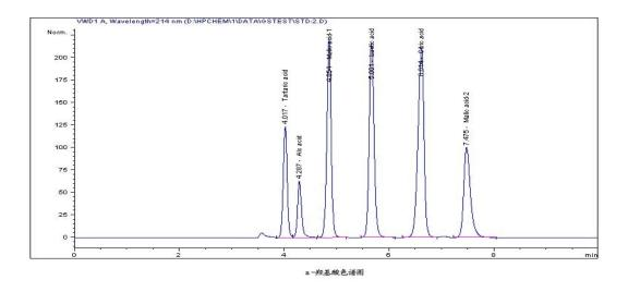
Fig. 1 - Standard liquid chromatogram of hydroxy acids
