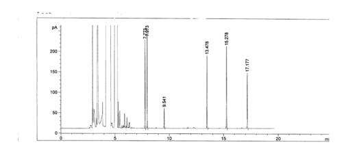
Fig. 3 Standard gas chromatogram of  $\alpha$ -hydroxy acids
