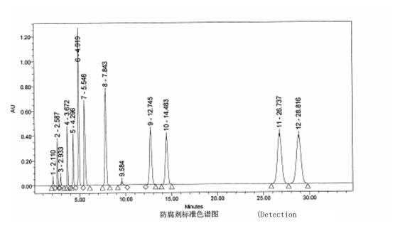
1: Methylchloroisothiazolinone (2.110); 2: 2-bromo-2-nitropropane-1,3-diol (2.587); 3: Methylisothiazolinone (2.933) 4: benzyl alcohol (3.672); 5: phenoxyethanol (4.296); 6: methyl 4-hydroxybenzoate (4.919); 7: benzoic acid (5.548); 8. Ethyl 4-hydroxybenzoate (7.843); 9: Isopropyl 4-hydroxybenzoate (12.745); 10: Propyl 4-hydroxybenzoate (14.483); 11. Isobutyl 4-hydroxybenzoate (26.737); 12:Butyl 4-hydroxybenzoate (28.816)
