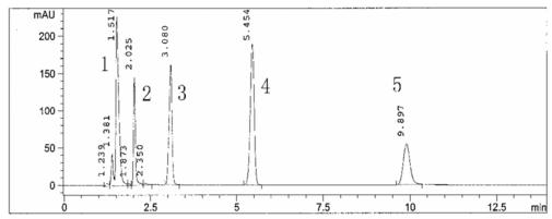
Fig. 1 Standard chromatogram of a crumb remover with a detection wavelength of 230 nm 1: Salicylic acid (1.517); 2: --; 3: Ketoconazole (3.080); 4: Clomiprazole (5.454); 5: Piroctone ethanolamine salt (9.897)
