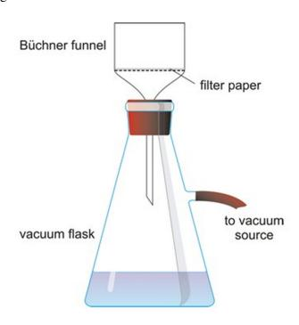
Figure 2: Simple vacuum filtration diagram. Source: https://glossary.periodni.com/glossary.php?en=vacuum+filtration
