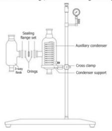
For the **SE13 / 5L** model that comes without an auxiliary condenser, connect the three-way flask directly to the main condenser, using the same steps as described above.
