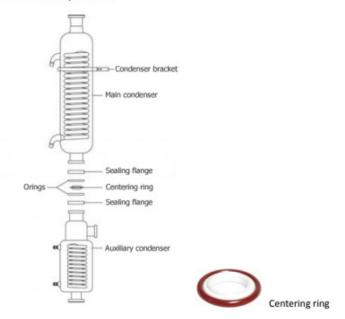
d. Identify all vacuum and chilling water connectors on the condenser (illustrated below is condenser for the 1.3G/5L model).
