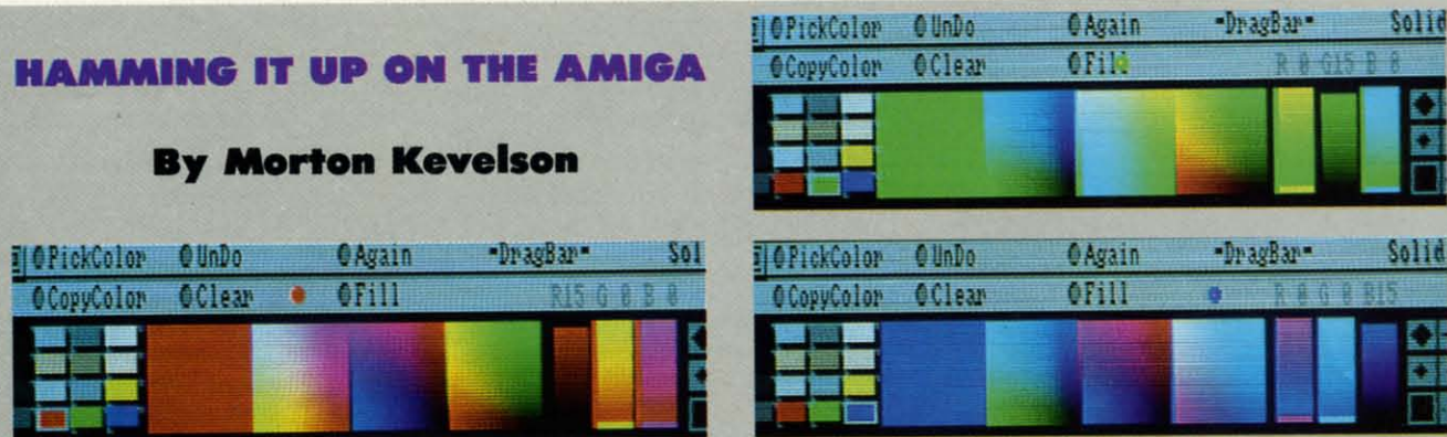
Shown are three views of Digi-Paint's color menu, used to illustrate the Amiga's 4096 color hold and modify display mode. At bottom left the base color is red, at top right it's green, and at bottom right we work with blue.
