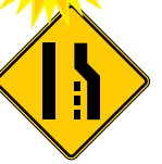
Pavement Width Transition Right S3030W42R(H)A S3636W42R(H)A
