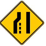
Pavement Width Transition Left S3030W42L(H)A S3636W42L(H)A
