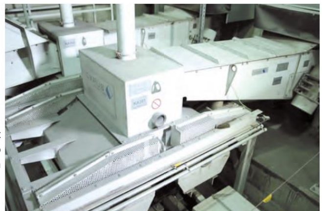
Image 3 (right): Chute distributor at the transfer point to the two main conveyor lines.
