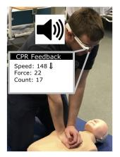
**Figure 5.10:** CPR Glass Assistant is providing instant feedback on compression depth (force) and speed while performing CPR
