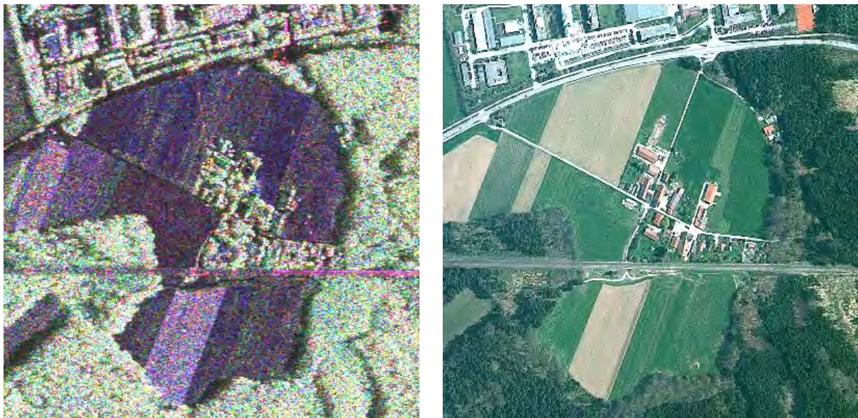
Fig. 2. Speckled polarimetric SAR image (left) and smooth panchromatic optical image (right), testsite Oberpfaffenhofen/Germany
