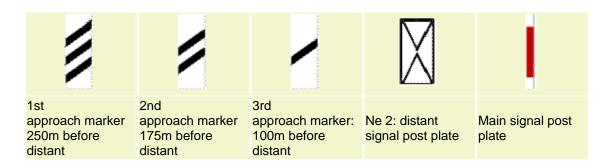
If a distant signal is mounted on one post with main signal, the approach markers and distant signal sign are not used, only the main signal post plate will be at the signal's post. A signal may also be equipped with a speed indicator.
