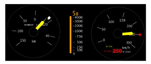
To the left you see the acceleration/deceleration meter, to the right you see the speed gauge. The speed gauge shows three speeds:
