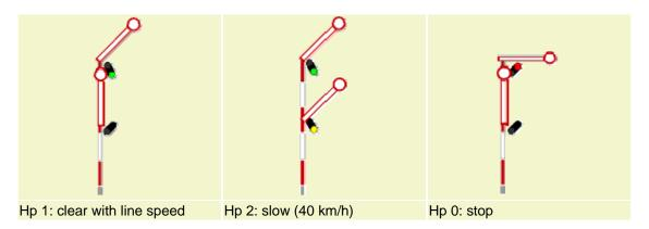
The signals are also equipped with lanterns that are lit at night, by gas lanterns in the old days, now by solar-driven LED matrices.
