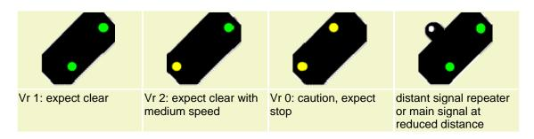
When a distant signal is in a reduced distance to the corresponding main signal, it carries a white light on the upper left edge.
