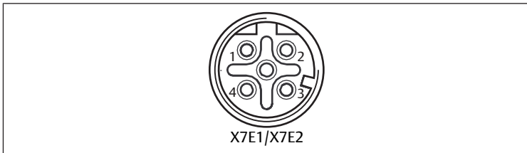
Fig. 3: Fieldbus connection pin assignments
